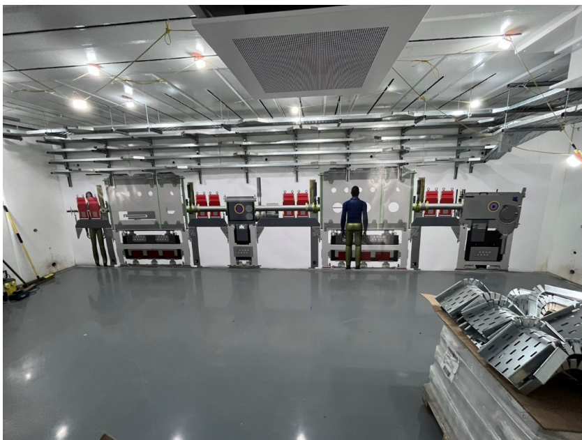
FEBE hutch showing layout of the beamline. Beam from right to left, with laser mirror box to bring in the 100 TW class laser co-linear with the electron beam, first experimental chamber, laser mirror box to dump the laser, and second experimental chamber. The spectrometer dipole is installed in the main accelerator hall.
