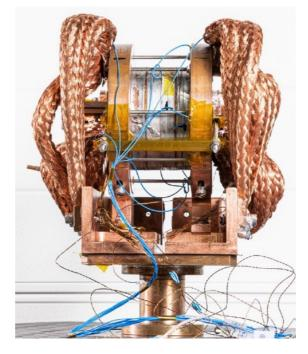
Figure 7. This solenoid test magnet is equipped with HTS coils and achieved a high field of 18 T at a temperature of 12 K in a 5 cm bore.
