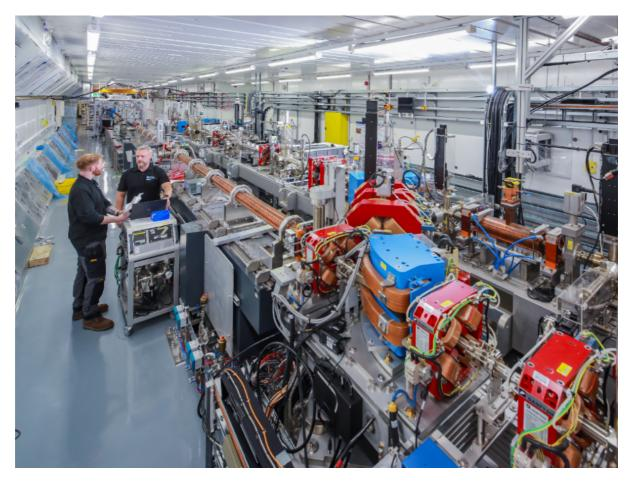
Figure 14. The CLARA upgrade to 250 MeV is now being commissioned at Daresbury Laboratory.
