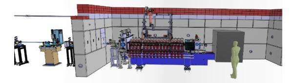
Figure 6. The planned P3 experiment at PSI uses the 5.8 GeV electron beam of SwissFEL to demonstrate high-yield positron production, albeit at low intensity. It uses a 12 T solenoid based on a non-insulated high-temperature superconductor, to maximise positron capture.
